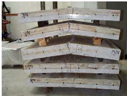
(b) Short slabs incorporating different ductility steels, tested with a central line load until fracture of steel reinforcement occurred
