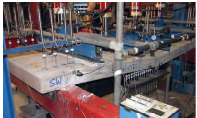
(b) Ringbeam being used in a SSOW test with fully restrained edges, and central cross-beam in (a) present.
