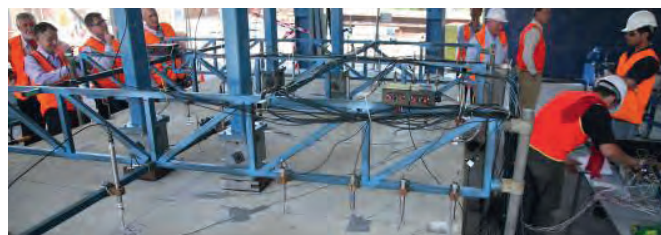
(b) Testing to failure using position-controlled jacks.
