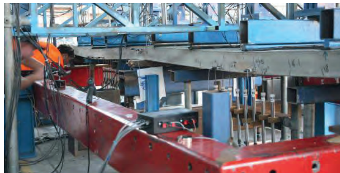
Figure 6. A DSOW slab test in progress.
