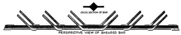
Kahn Trussed Bars (Kidder and Nolan, 1911)
