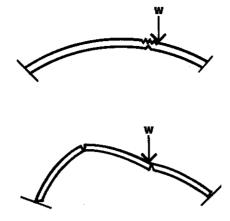
Figure 2 The failure of a masonry (voissoir) arch
