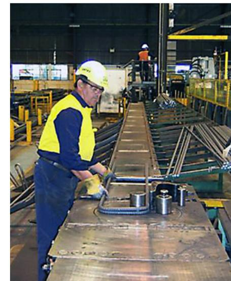
**FIGURE 4** *Factory Bending around Pins of Specified Diameters*
