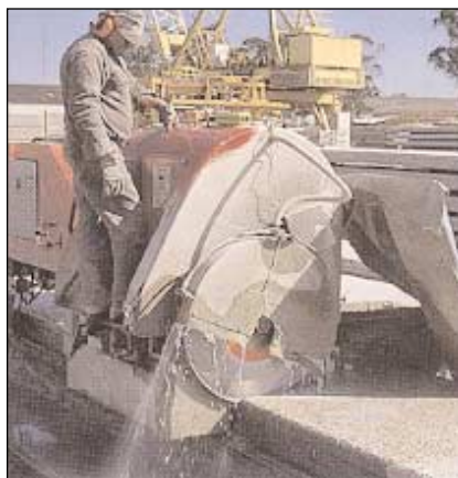
Panels being sawed to client's required length
