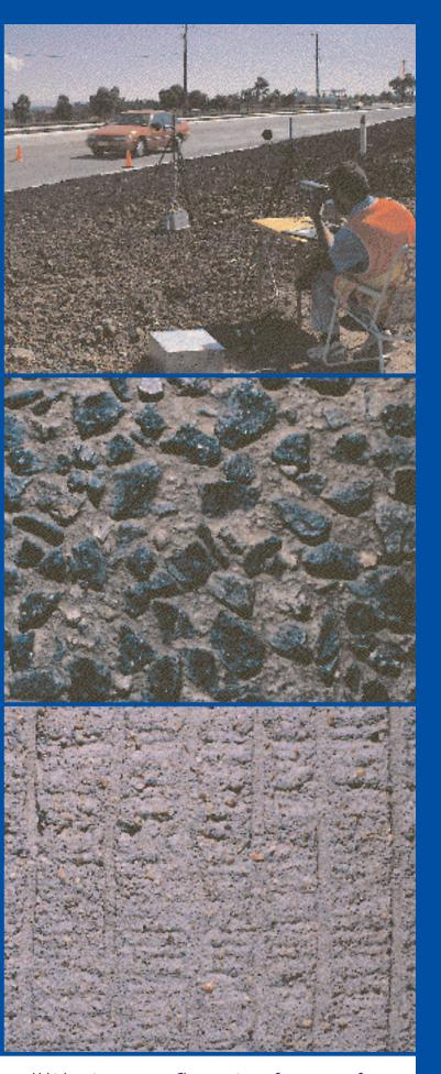
TOP: Vehicle noise measurement on Keilor Park Drive, Keilor Park, Victoria Close-up views of concrete surfaces — exposed aggregate (CENTRE) and a tyned surface (ABOVE)
