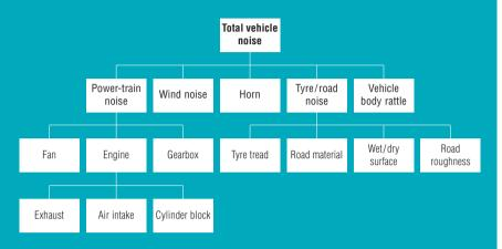
The total amount of traffic noise can be affected by factors such as the type of traffic (trucks or cars), traffic speed, accelerating and braking areas at intersections and the grading of the road. Australian road and traffic specialists have been actively involved in minimising traffic noise in urban areas by using techniques such as:
