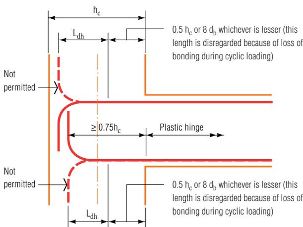
(b) Anchorage of beam bars when the critical section of the plastic hinge forms at the column face (from NZS 3101: Part 2:1995)
