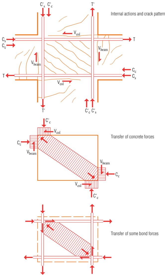
(a) Shear transfer of concrete compression forces and some bond forces from longitudinal bars by diagonal compression strut mechanism (from Goldsworthy<sup>9</sup>)
