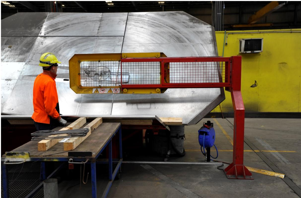
The mechanical properties of steel reinforcement change when a bar is bent or straightened from a feed coil (most small-diameter bar sizes up to 20 mm are supplied by coil). Similarly, when bars are welded together to make a sheet of mesh the mechanical properties of the final product have changed.
