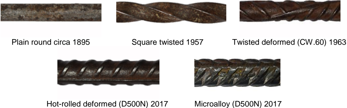
Figure 2 A chronology of reinforcing bar types
