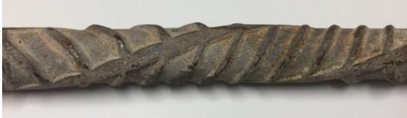
**Figure 9. Cold-twisted deformed bar (CW.60) 1963**
