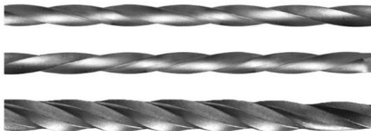
**Figure 7. Single and Twin-twisted square bars**
